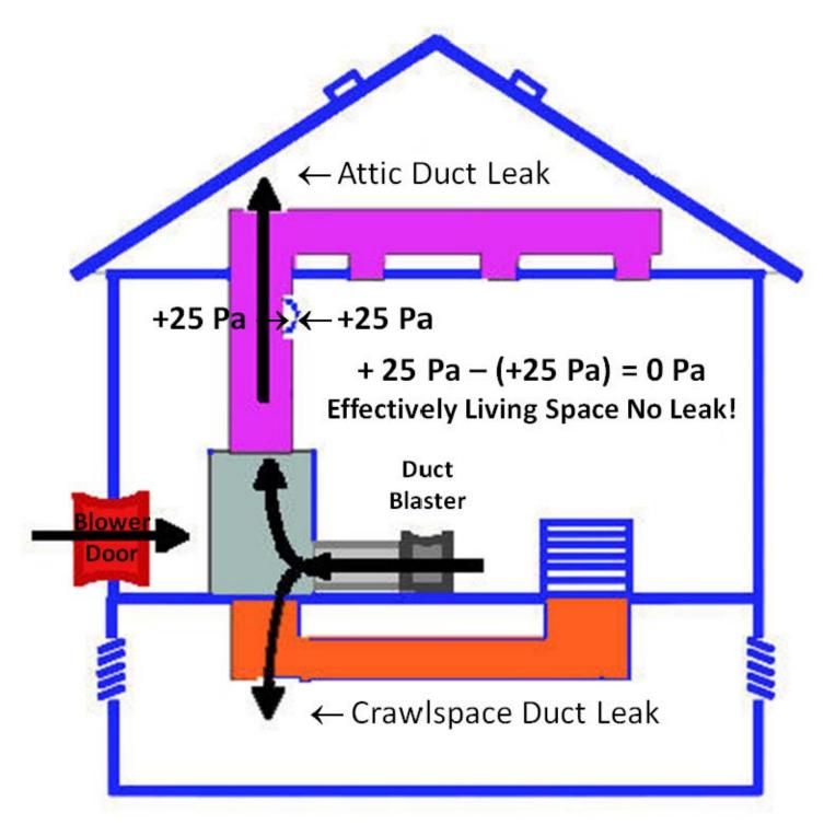
The goal is to determine the amount of duct leakage lost outside the house. Duct leaks may prevent delivering air where wanted in the house, but the energy itself stays in the house.
